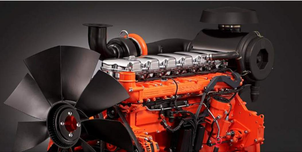
The engines for power generation from Scania are based on a robust design with a strength optimised cylinder block containing wet cylinder liners that can easily be exchanged. Individual cylinder heads with 4 valves per cylinder promotes repairability and fuel economy.
